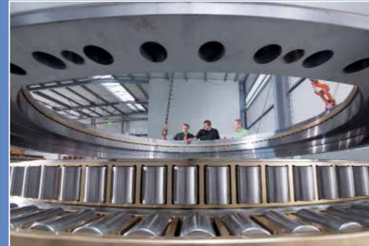
Three-row roller bearing with closed brass cages used as main bearing for a shaftless direct driven 5 MW wind turbine.
