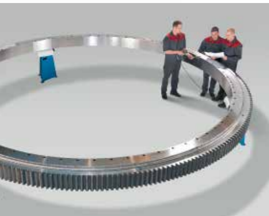
Large shipboard crane with a Triple Row external toothed Roller Slewing Ring. The high load capacity and compact proportions of this type of Slewing Ring are ideally matched to the mast and base block proportions of the crane.
