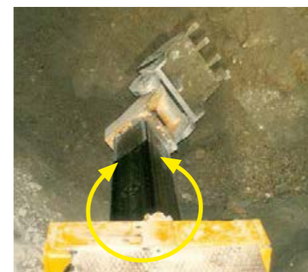
Slew Drive SP-HC 0698 with hydrostatic gear for turning an excavator boom, part of a cutter bar.
