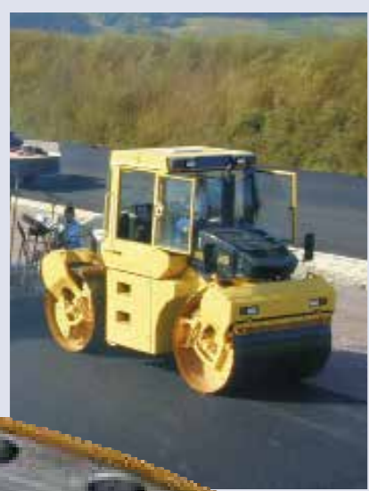
Tandem asphalt compaction rollers use untoothed Slew Rings as a steering bearing (some designs are partly coated on the surface to prevent corrosion). In the split roller, Slew Rings with special seals are used.
