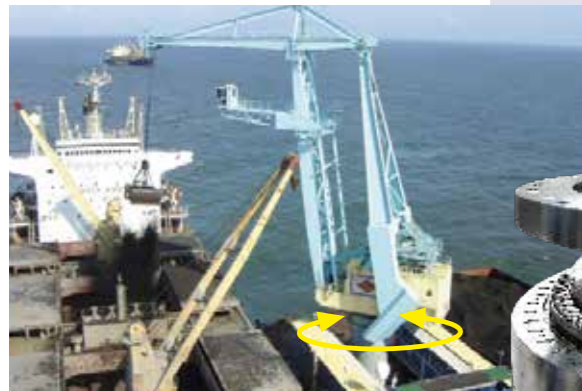
Harbour pontoon crane
