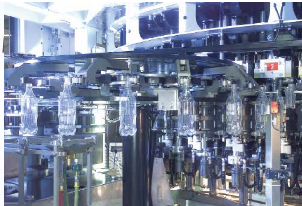
Precision Single Row Ball Slewing Rings with cages are used for the rotating carousels in fast running blow moulders for the production of polyethylene PET bottles. Such Slewing Rings run continuously and reliable service life is an essential design criterion.
