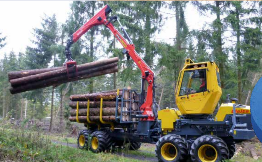
Slewing the grapple of this forwarder is done by means of a Slew Drive series SP-I.
