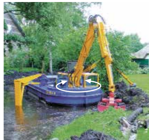
This work boat which is used in Dutch canals is fitted with a WD-L series Slew Drive to move the boom of the excavator.
