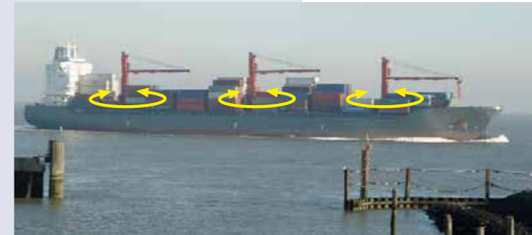
Shipboard cranes on container vessels use internal toothed Triple Row Roller Slewing Rings. The examples in this photograph are fitted with Slewing Rings that are 2,650 mm (104 in) in diameter and carry tilting moments up to 15,000 kNm (11,063,983 ft-lb).
