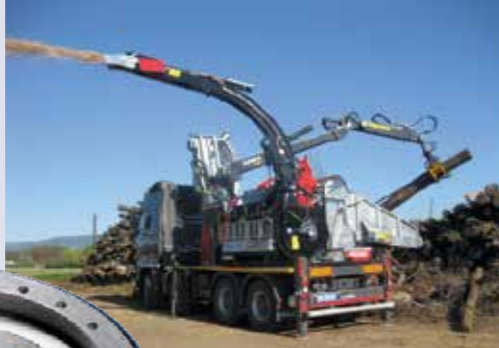
Slew Drives series WD-L and SP-I are used by these wood-choppers to position the chipper and the expulsion tool as well as to maneuver the grapple.
