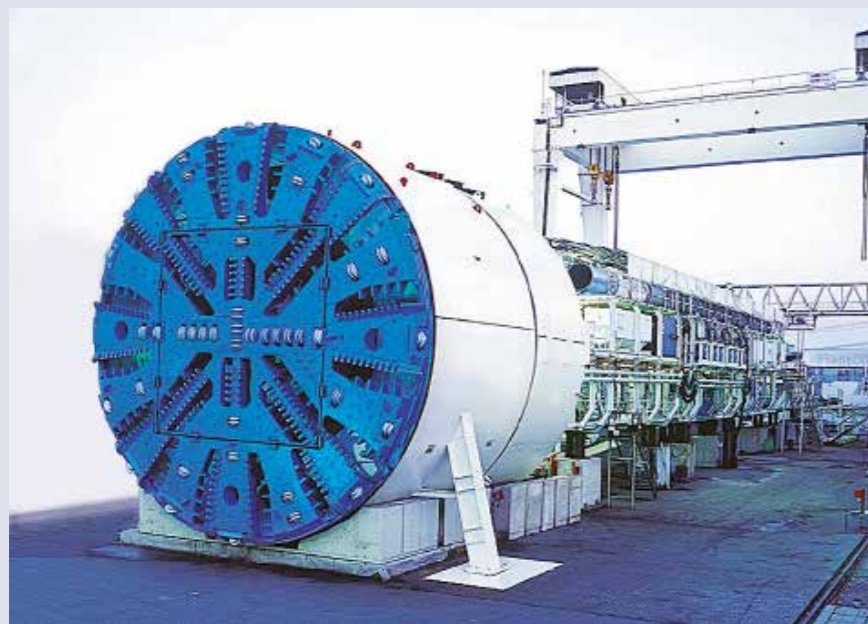
Tunnel boring machines use large and heavy Triple Row Roller Slewing Rings in cutting heads.
