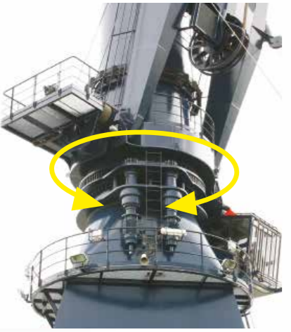
Large shipboard crane with a Triple Row external toothed Roller Slewing Ring. The high load capacity and compact proportions of this type of Slewing Ring are ideally matched to the mast and base block proportions of the crane.
