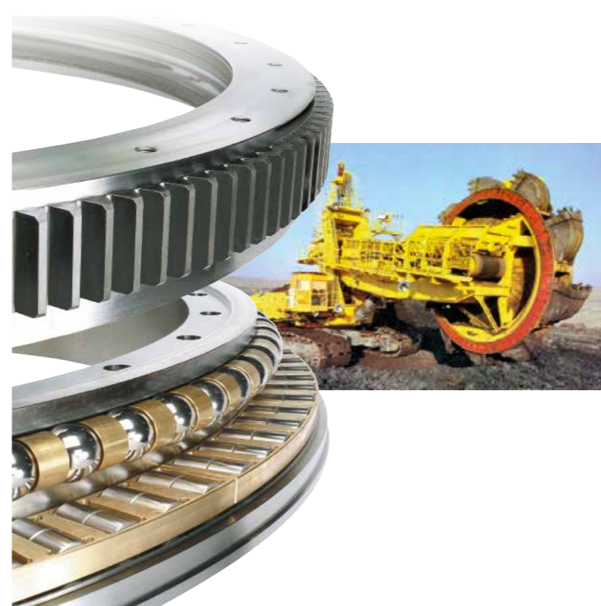
Cross section of a typical main Slew Ring. This unit is a combination type with external tothing and a diameter of 4,800 mm (189 in).
