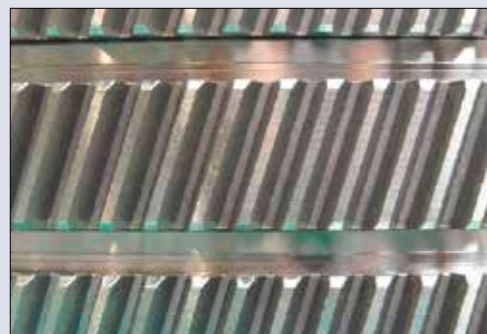
External helical gear, normalized
