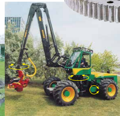
Harvesters use our Ball Slewing Rings and Slew Drives for the axle swing arm, the crane boom, the harvester head (with a chain saw) and a rotatable cab.
