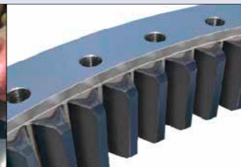
Quenched and tempered ring, induction hardened wear resistant tooth flanks
