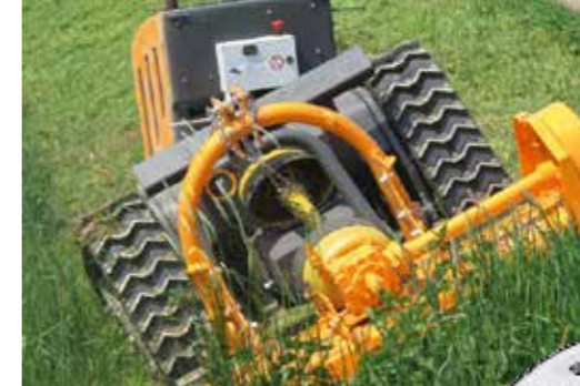
These flail mowers rely on Slew Drives series WD-L to position the mower.
