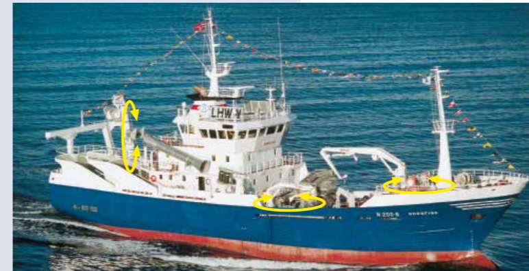
Deep sea fishing vessels use Ball Slewing Rings for shipboard cranes and net handling equipment. Typical external diameters range between 600 to 1,500 mm (23,6 to 59 in).
