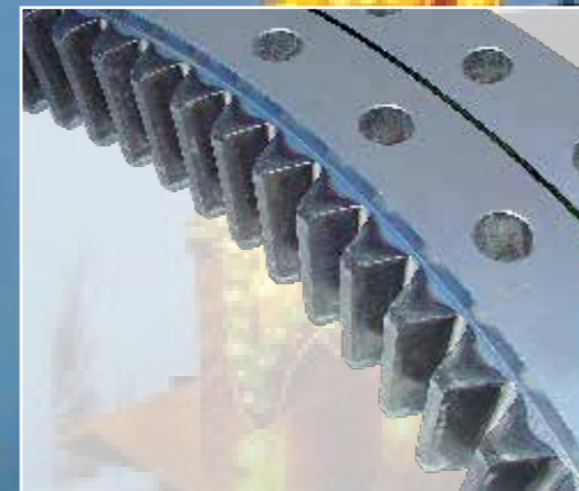
"Tango" is one of the most breathtaking amusement park rides in its class. Each gondola is driven in its three rotational axes via five Slew Rings which have adv internally hardened toothing.
