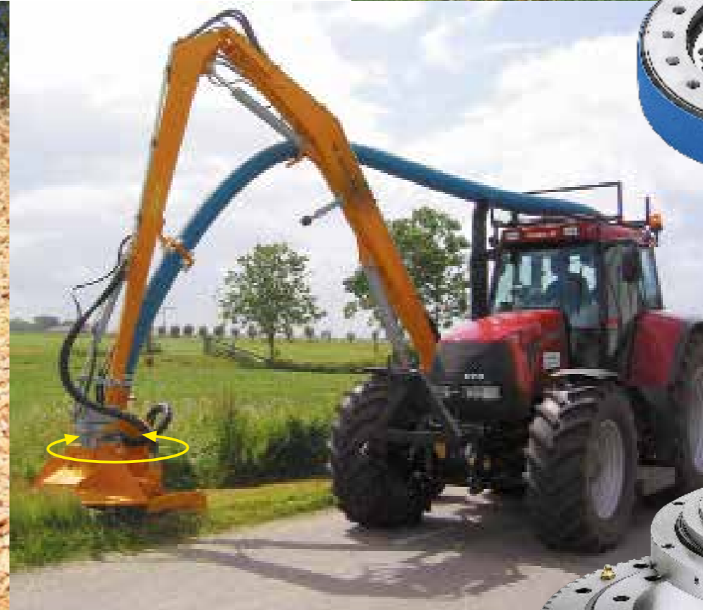
These flail mowers rely on Slew Drives series WD-L to position the mower.
