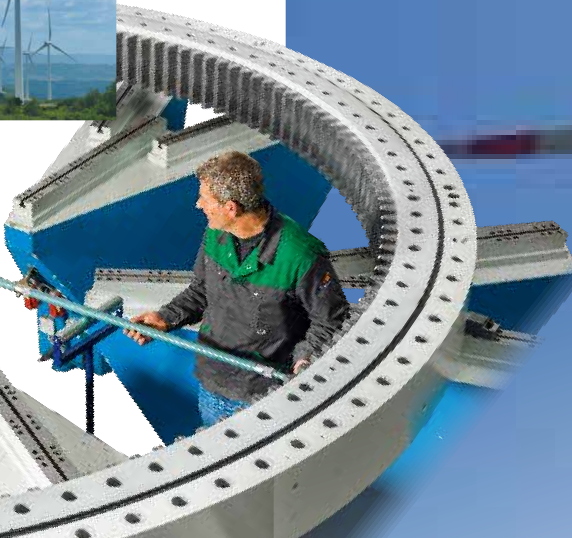
Measuring the gearing of a blade bearing used in a 7 MW Offshore turbine with a ball diameter of 80 mm, an outer diameter of around 5 m and a total weight of 8000 kg.
