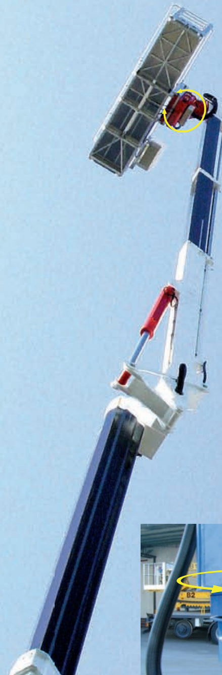
This working platform with a height of 35 m uses two IMO Slewing Rings on a synchronous rotating turntable which are driven by an IMO WD-HC 0146 Slew Drive.
