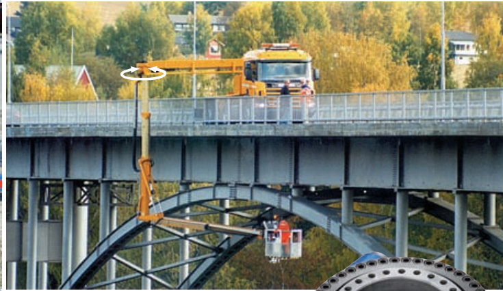
This bridge inspection equipment uses Slew Drive WD-HC 0300 in the boom joint. The unit is able to accommodate the suspended loads and is fitted with a worm drive and multi-plate disk brake.
