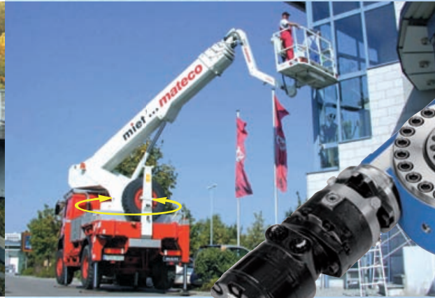
This working platform with a height of 35 m uses two IMO Slewing Rings on a synchronous rotating turntable which are driven by an IMO WD-HC 0146 Slew Drive.
