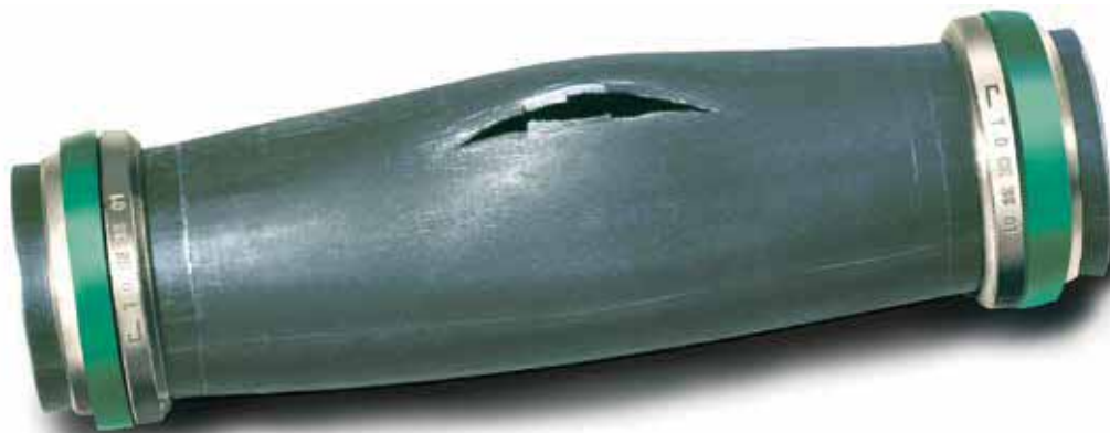
Destructive testing with 28x2 carbon steel tube. The tube burst at 650 bars without any leakage or sweating from the sealing points.
